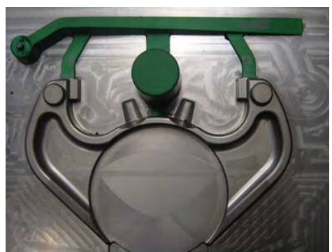
Figure 7. Photo of revised pattern with single feeder.
