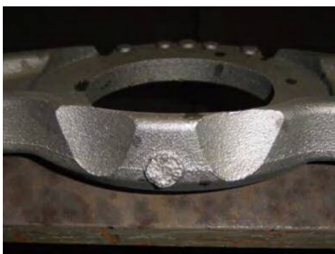
Figure 8. Photo of the contact area with a single feeder.
