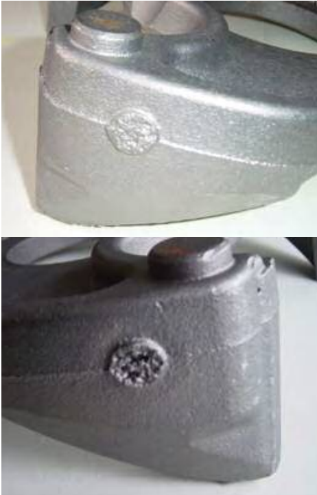
Figure 3. Feeder contacts with original design (2 feeders).
