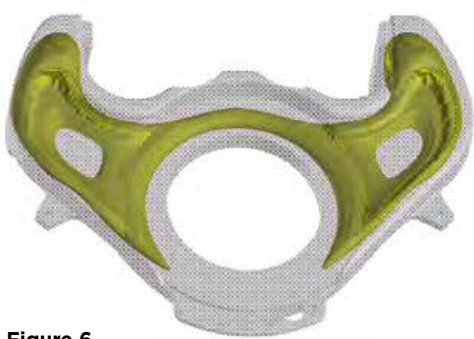
Figure 6. Plot of transfer modulus of 0.645 cm in the casting.
